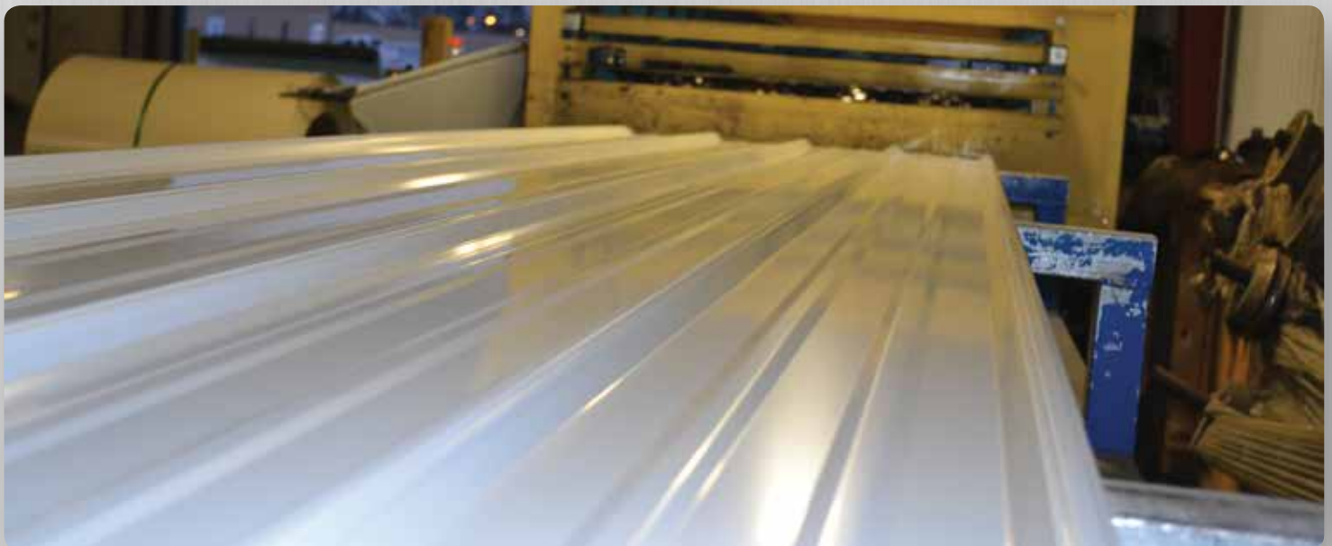
Corrugated sheet metal exits the form roller to become siding and roof panels on our buildings.
