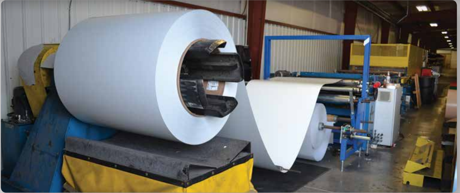
Painted metal coils unroll and are directed towards a form roller.
